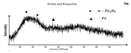
Fig. 1. XRD pattern of Ferric Nanoparticles deposited by CBD method.
